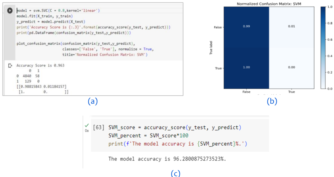
Figure 3. Calculations using the linear kernel: (a) Create model with Linear Kernel; (b) Confusion Matrix plot for Linear Kernel; (c) Accuracy Result for Linear Kernel
