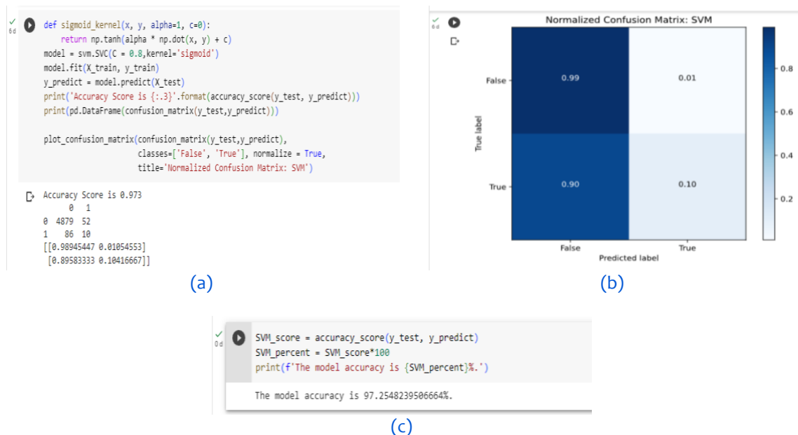
Figure 6. Calculations using the Sigmoid kernel: (a) Create Model with Sigmoid Kernel; (b) Confusion Matrix plot for Sigmoid kernel; (c) Accuracy Result for Sigmoid Kernel
