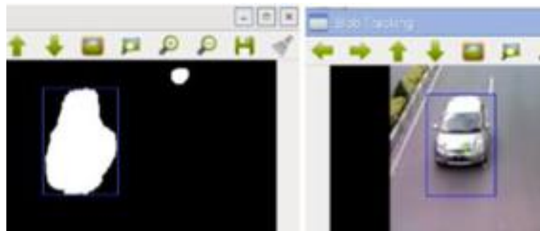
Figure 2. Object Detection Using BLOB Tracking
