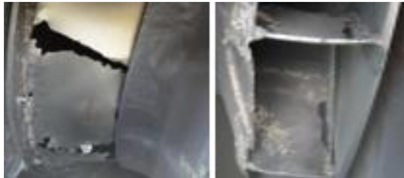
Figure 1. Damage to IDF fan blade and cone
