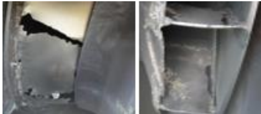
Figure 1. Damage to IDF fan blade and cone
