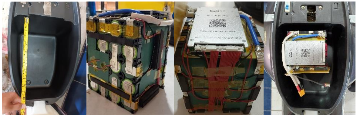
Figure 2. LFP with Smart BMS assembling
