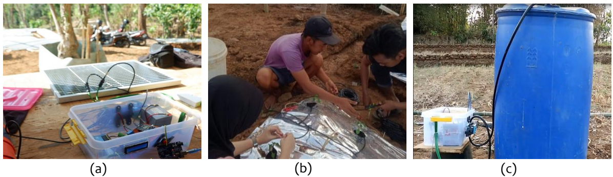
Figure 5. (a) Preliminary evaluation of the equipment; (b) Drip irrigation installed on agricultural land; (c) Testing of equipment on agricultural land
