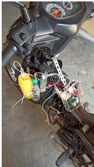
Figure 2. The application of the electrolyzer on a motorcycle
