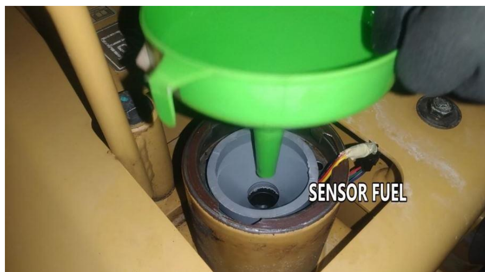
Figure 3. Refueling of the unit using the smart monitoring device
