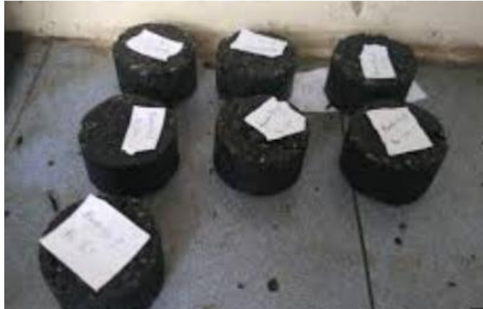
Figure 4. Asphalt after soaking
