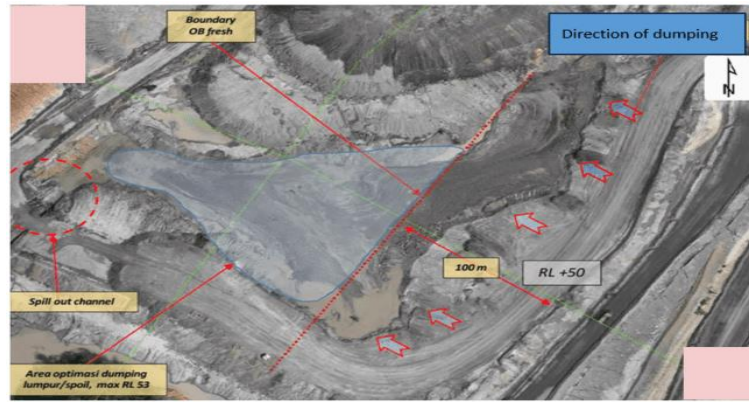
Figure 1. Operating procedures of mudcell[10]
