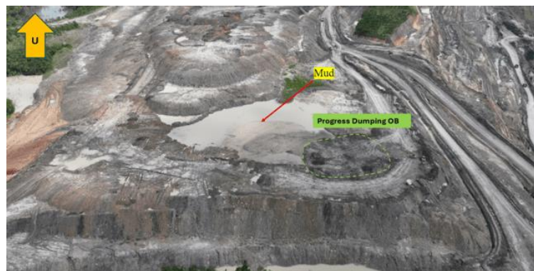
Figure 2. Progress of Dumping Overburden in mudcell[11]
