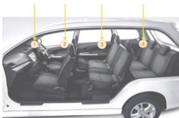
Figure 2. Placement of the temperature sensor in the cabin
