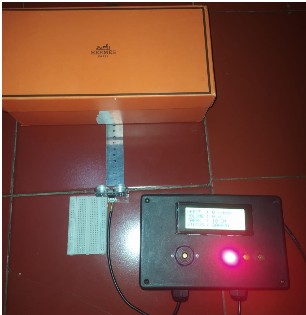
Figure 3 . Ultrasonic sensor testing detecting solid objects
