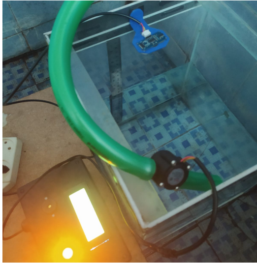
Figure 4. HC-SR04 ultrasonic sensor testing when detecting water level distance
