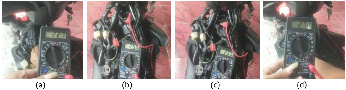
Figure 5. Voltage measurement data capture; a). Without flash cable, b). Flash cable 11 coils, c). Flash cable 16 coils, d). Flash cable 21 coils
