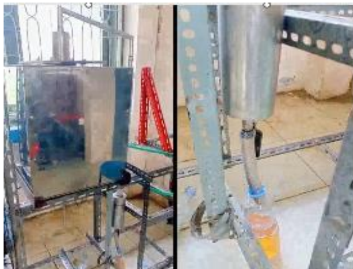
Figure 5. Running pyrolysis equipment
