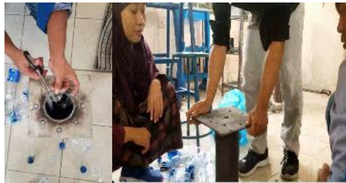
Figure 3. Inserting plastic into the reactor
