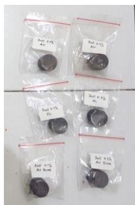
Figure 3. The results of the circulating quenching test samples.
