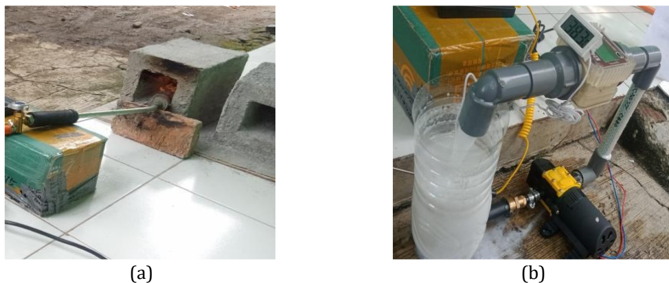
Figure 2. (a) heating device, (b) circulating quenching device.
