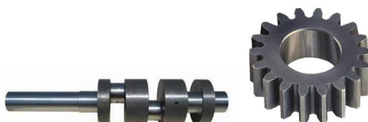
Figure 1. Application of AISI 4140 to crankshaft and gear.
