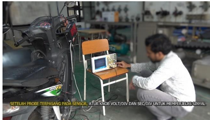
Figure 6. Instal probe on o2 sensor and parameter settings (oxygen sensor measuring)
