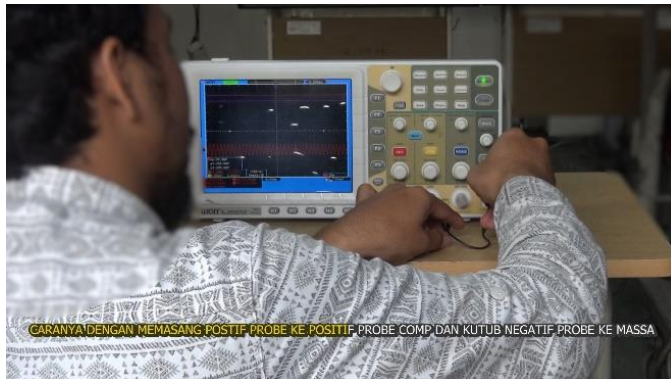
Figure 4. Ignition and autoset process
