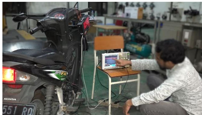
Figure 7. Analysis of O2 sensors signals (oxygen sensor measuring)
